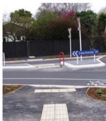
Photo 15.18 – Crossing point by roundabout, St Albans, Christchurch (Photo: Tim Hughes)
