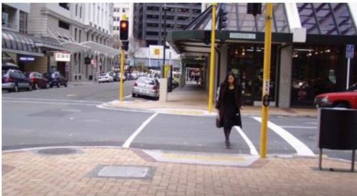
Photo 15.15 – Use of kerb extensions maintains straight continuous accessible path, Featherston St, Wellington (Photo: Tim Hughes)
